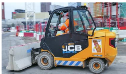
Figure 22: Electric telehandler with load
