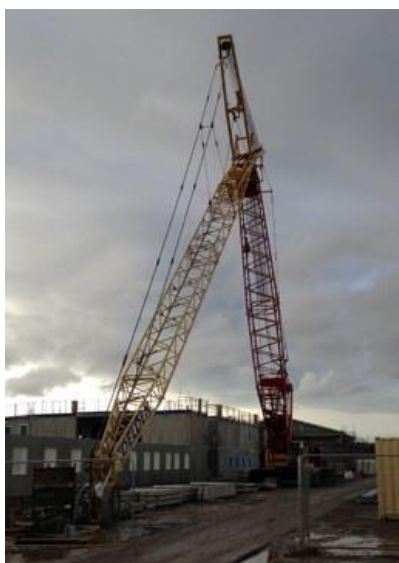
Figure 21: crawler crane rigged with luffing jib
