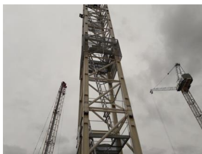
Figure 15: Tower crane with anti climb panel
